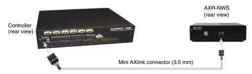
FIG. 7 AXR-NWS connection to a Controller
